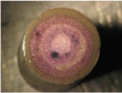
FIGURE 5. Cross Section of 5-Layered Extrudate. Left: Perpendicular to Extrusion Direction; Right: Parallel to Extrusion Direction.
