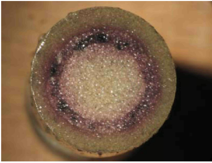
FIGURE 4. Cross Section of 3-Layered Extrudate. Left: Perpendicular to Extrusion Direction; Right: Parallel to Extrusion Direction.
