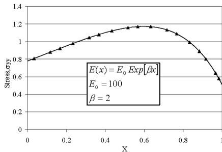
FIGURE 5. Comparison of Finite Element and Exact Solution for Functionally Graded Bar under Tension
