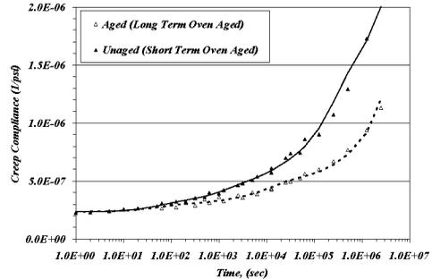
FIGURE 4. Creep Compliance Master Curves with Fitted Generalized Kelvin Model (markers indicate laboratory data and lines show fitted models)
