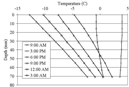
FIGURE 2. Temperature Variation through the Depth of Asphalt Concrete Pavement
