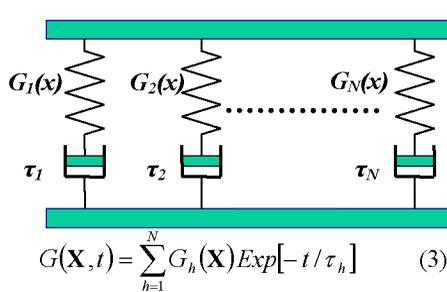
FIGURE 3. Generalized Maxwell Model
