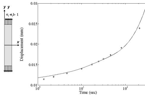
FIGURE 6. Comparison of Finite Element and Exact Solution for Viscoelastic Bar under Tension
