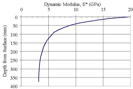
FIGURE 1. Aged Asphalt Concrete Properties after Two-Years in Service
