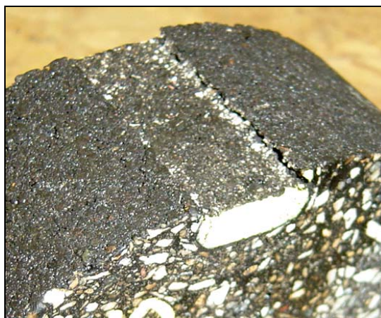
Figure1 - Crushing Failure under Regular IDT Loading Head (Mix-40)
