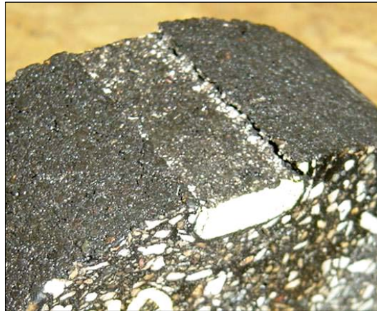
Figure 2. Crushing under loading heads.
