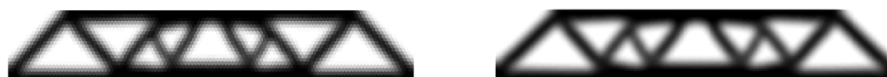
Figure 4. MBB beam design with projection scheme and Wachspress hexagonal element. Note that the designs with coarse mesh (left) and fine mesh (right) are identical unlike the other two approaches.
