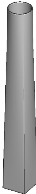
Figure 3. Design domain (outer skin or shell) for topology optimization of a building
