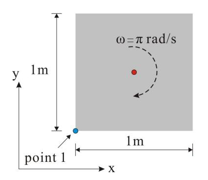
Mass density:  $\rho = 1.0 \text{ kg/m}^3$ Young's modulus: E1=10Mpa; E2=1Mpa; E3=0.5Mpa Poisson's ratio:  $\nu=0$ Thickness: h=0.1m
