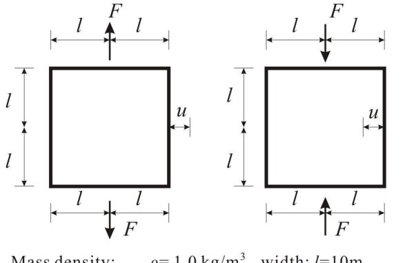
Mass density:  $\rho = 1.0 \text{ kg/m}^3$  width: l=10mYoung's modulus: E=10pa Poisson's ratio: v=0 14
