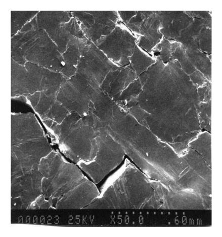
Fatigue fracture along the interface between crystals in a metal http://www.larrylawson.net/fatigue.htm
