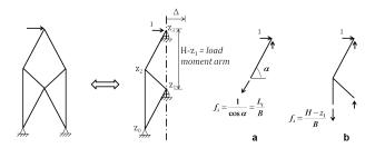
the forces in the diagonals are  $f_i = \frac{L_i}{B}$  while the forces in the columns are given by  $f_i = \frac{(H-z_i)}{B}$ . The displacement at the top of the frame is
