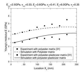
Fig. 6. Comparisons of effective FGM Young's moduli between the proposed model simulations and experimental data [31].
