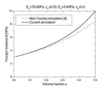
Fig. 4. Comparisons of effective glass-epoxy FGM Young's moduli between the proposed model simulations and Mori–Tanaka method [6].
