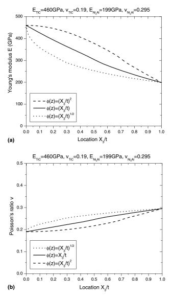
Fig. 3. Effect of phase volume fraction distribution on (a) the effective FGM Young's modulus and (b) the effective FGM Poisson's ratio.
