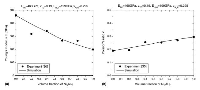
Fig. 7. Comparisons between the proposed model simulations and experimental data [30]; (a) the effective FGM Young's modulus vs. phase volume fraction and (b) the effective FGM Poisson's ratio vs. phase volume fraction.
