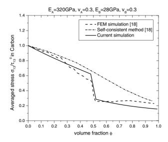
Fig. 5. Comparisons of averaged shear stress distribution among the proposed model, self-consistent method [18], and finite element method (FEM) [18].
