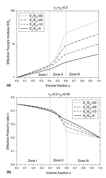
Fig. 2. Effect of modulus contrast ratio on (a) the effective FGM Young's modulus and (b) the effective FGM Poisson's ratio.
