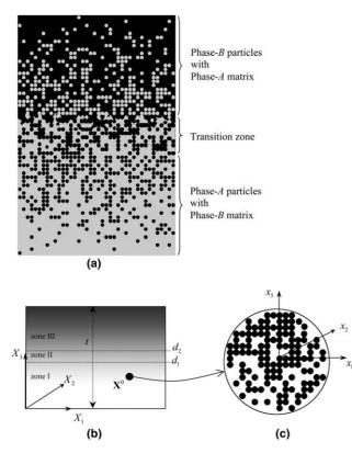
Fig. 1. Schematic illustration of a two-phase FGM sample: (a) typical microstructure including A and B phases; (b) three zones in macroscopic scale X; and (c) RVE in the microscopic scale x.
