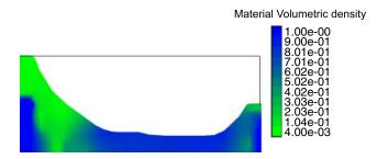
Plate 1. Material distribution for the FG turbine disk.
