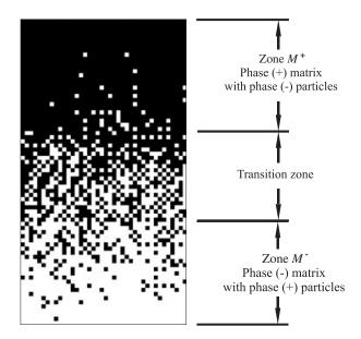
Figure 1. Schematic representation of an FGM.
