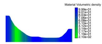
Plate 3. Material distribution considering x-direction gradation for the FG turbine disk.
