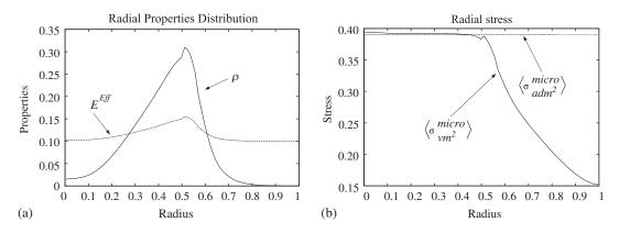
Figure 6. Material and Von Mises stress distribution along the radius of the FG rotating disk.
