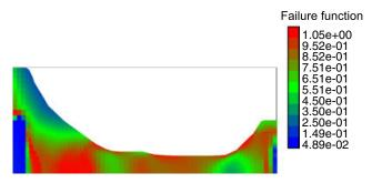
Plate 2. Failure function of the FG turbine disk-see Equation (23).
