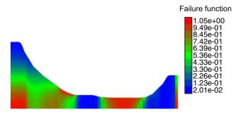
Plate 4. Failure function considering x-direction gradation for the FG turbine disk—see Equation (23).
