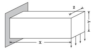
Figure 6. Design problem: finding optimal material distribution in a hexahedron with the left end fixed and a distributed load applied on the right bottom edge (X:Y:Z = 3:1:1).
