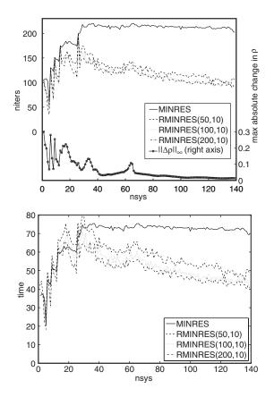
Figure 9. Number of iterations (niters) and time (s) of RMINRES(s, k) with fixed k = 10 and varying s.
