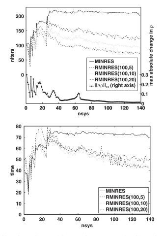
Figure 10. Number of iterations (niters) and time (s) of RMINRES(s, k) with varying k and fixed s = 100.
