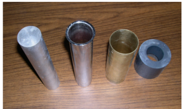
Fig. 2. A set of molds for making layered feedrod.
