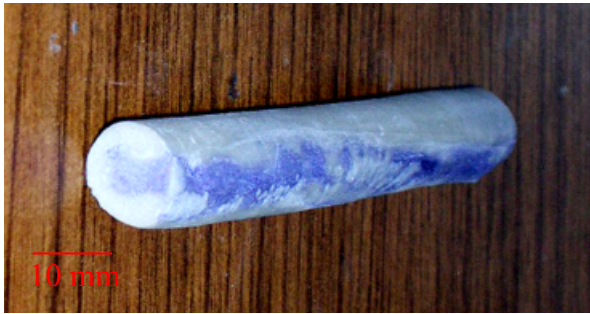
Fig. 10. Tangling of two layers due to unmatched rheology. Diameter = 12 mm.
