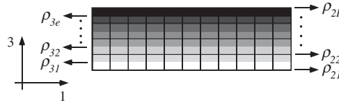
Figure 8. Piezoceramic design domain divided into horizontal layers. Design variables \rho_{2J} and \rho_{3e} are defined for each layer interface and each layer, respectively.
