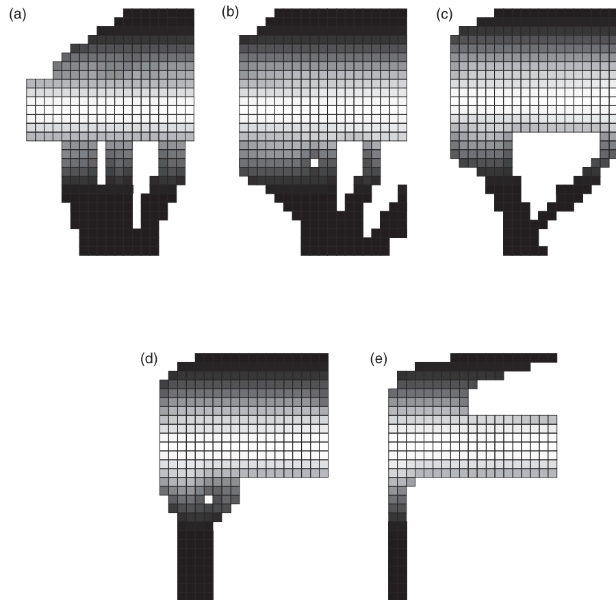
Figure 13. Detail of the piezoactuator ends shown in Figure 12: (a) w=0.5 , (b) w=0.6 , (c) w=0.7 , (d) w=0.8 , (e) w=0.9 .
