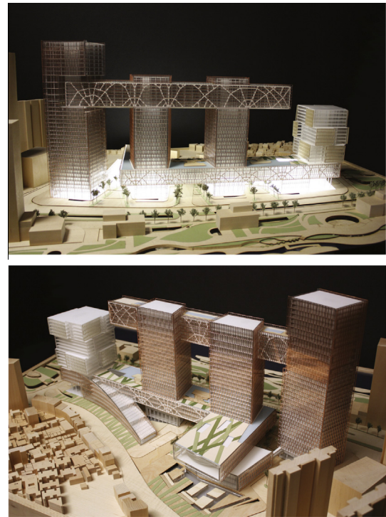
Fig. 7. Picture of the physical model for the concept design of the Zendai competition using topology optimization results.
