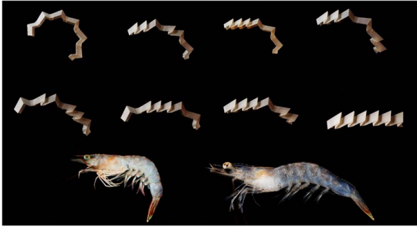
Fig. 1 Various stable states of a multi-stable Shrimp pattern tessellation, which has a segmented structure similar to arthropods such as shrimps. This curved design is a generalization from the standard Shrimp pattern, whose geometry is elaborated upon in Appendix A.
