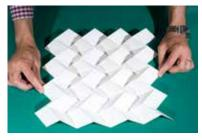
A comparison between the second and third figures shows that the material exhibits a negative Poisson's ratio – meaning it dilates when stretched.
