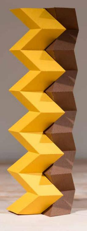
Two structures paired in the "zippered tube" configuration are stiff enough to hold weight, yet can return to their flat states for easy shipping or storage.
