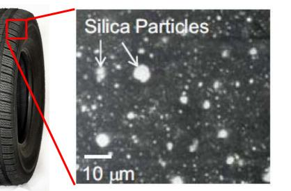
Microstructure of a typical filled elastome (Ramier, 2004)
