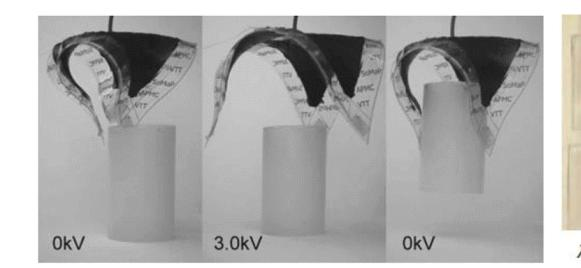
Finite deformation of a dielectric elastomer (Kofod, Wirges, Paajanen Bauer, 2007)
