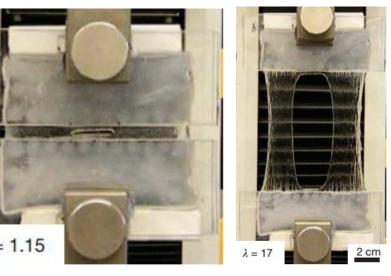
Stretch of a hydrogel specimen (Sun et. al., 2012)
