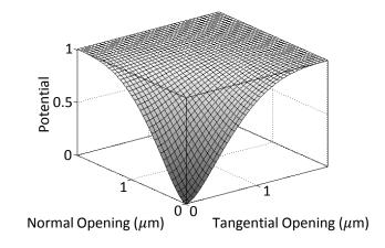
From the cohesive potential, one can determine the traction-separation relations by taking the respective derivatives
