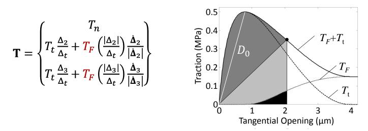
The above model is general. However, the newly proposed friction model is designed to be coupled to the PPR cohesive model, and adjusts as the cohesive model adjusts:
