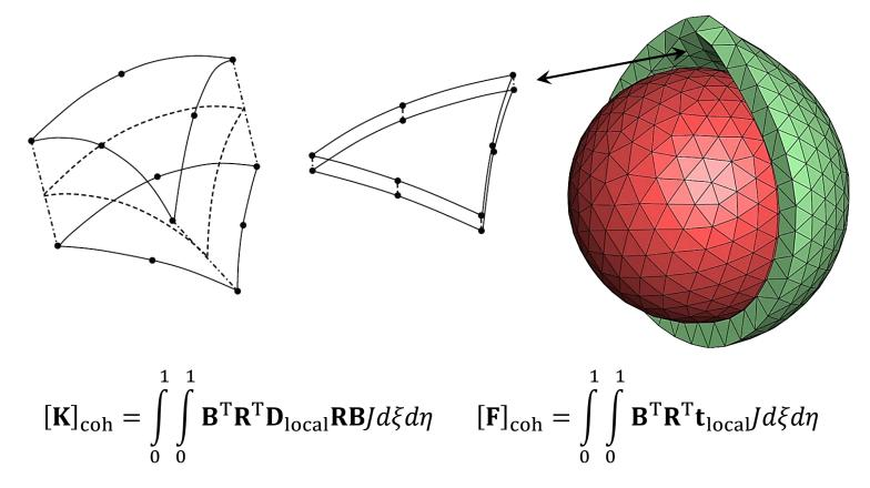
The cohesive elements are implemented as a user defined subroutine in a commercial software package<sup>1</sup>.
