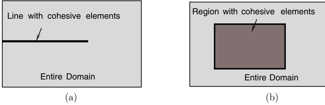
Figure 4.1: Generation of cohesive elements (a) along a straight line; (b) within a box region
