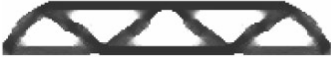
Figure 15 : Result extracted from reference [22], which illustrates that the monotonicity based length scale method leads to problems at corners.
