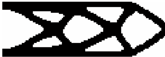
(b) Cantilever beam is solved with 120x40 elements and r_{\min} = 3.0 : gray structural members disappear.
