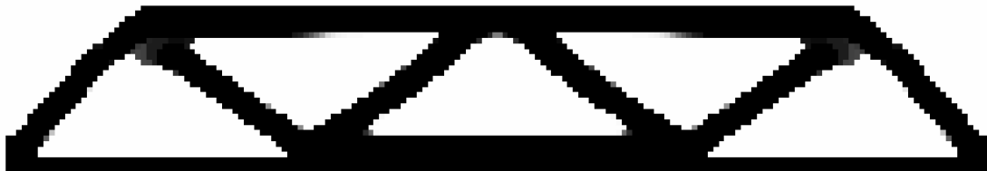
Figure 16 : Beam example using the new approach: minimum member size is 20% of the beam height; volume fraction is 45%; Poisson's ratio is 0.3; and penalization is 3 without continuation. The discretization (180x30 Q4 elements) is the same as the one in Figure 15.
