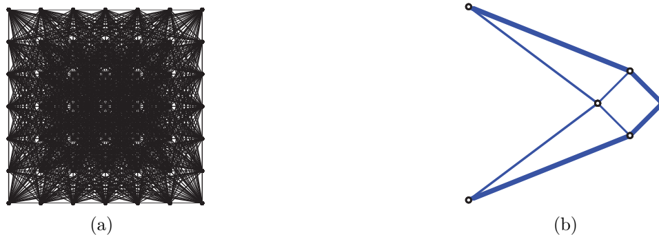
Figure 1.4: Generation of ground structure for full level connectivity: (a) initial ground structure; (b) optimal topology.
