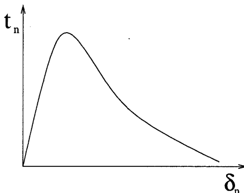
Figure 1.10: A schematic drawing of a cohesive law in terms of normal opening displacement ( \delta_n ) and normal traction ( t_n ).
