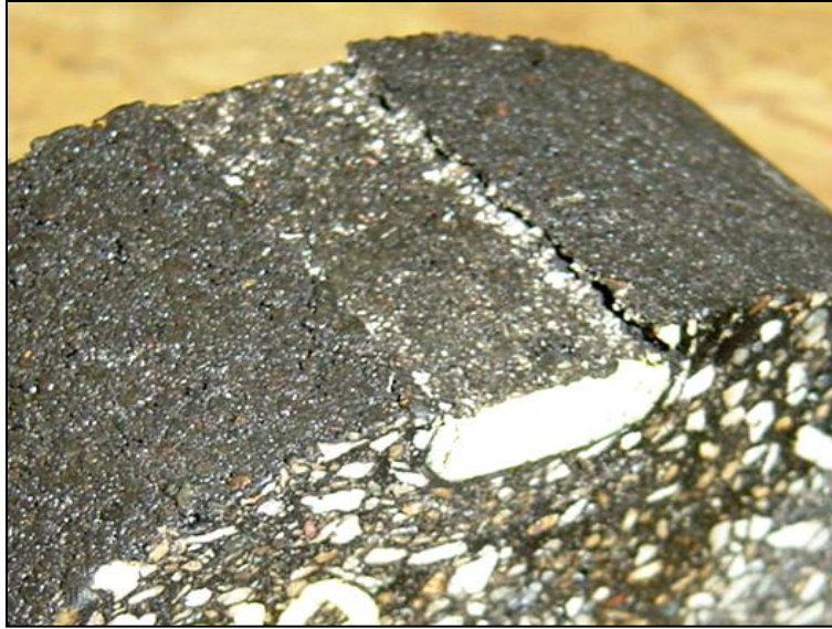
Figure 3-3: Crushing Under the Loading Head
