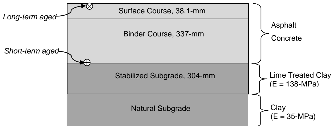
Figure 6-6: Full-Depth Asphalt Pavement Section (I-155, Lincoln, IL)
