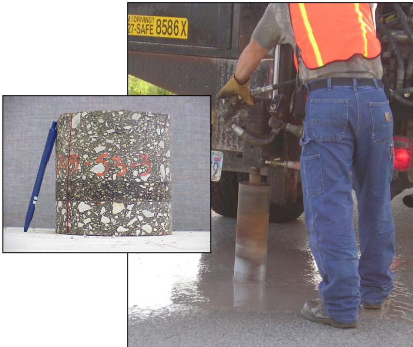
Figure 3-1: Field Core Sample Procurement (inset: Cored Sample)
