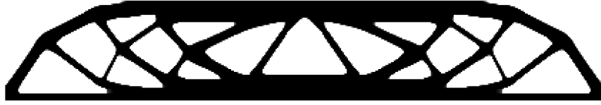
Figure 3.7: Solution to the MBB beam problem using total variation regularization and the forward-backward splitting algorithm
