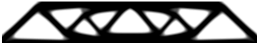
Figure 4.4: Final density field for the MBB problem and \beta = 0.06 plotted in grayscale. This result was generated using the TMP algorithm with \tau_0 = 2 and m_n = 1
