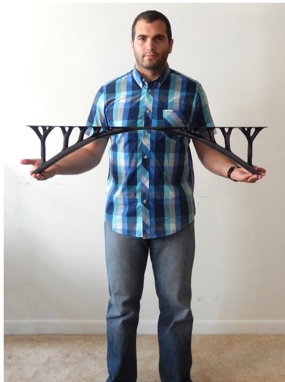
Figure 7.1: Author holding a 3 foot-long manufactured bridge obtained with density-based topology optimization using SIMP. The bridge is made from 3 pieces of 1 foot-long pieces.
