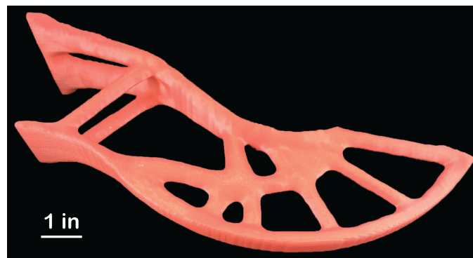
Figure 5.18: A printed model of the serpentine design using the FDM 3D printing.
