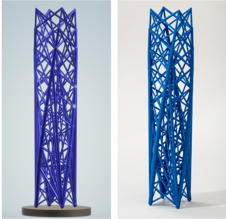
Figure 6.12: Comparison of the optimized twisting tower (left) and its printed model (right) using FDM process.
