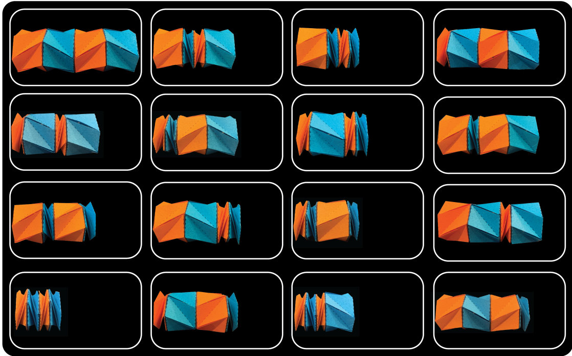
Figure 5.1: The sixteen stable states of a four-cell Kresling assembly.
