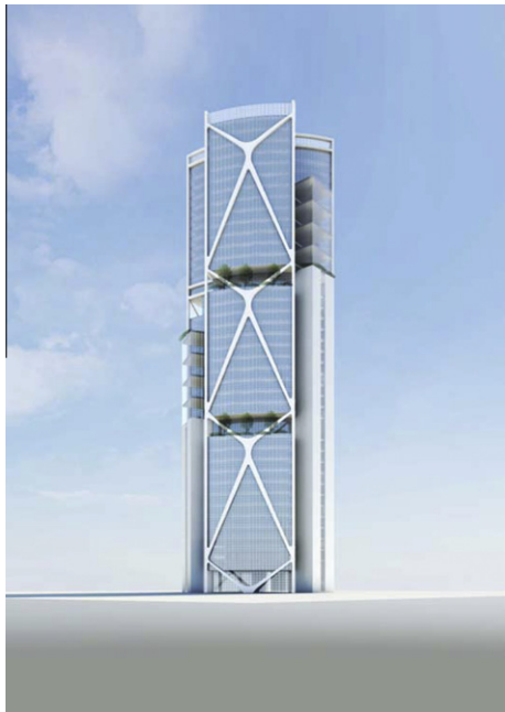
Fig. 14. Rendering of a competition entry showing an optimal bracing system (image courtesy of Skidmore, Owings & Merrill, LLP).
