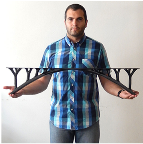
Fig. 20 Three foot long bridge obtained with density-based topology optimization using SIMP (scaled version of the result in Fig. 16b). The bridge was split into 3 pieces, 1 foot long each, manufactured using an FDM process and assembled afterwards
