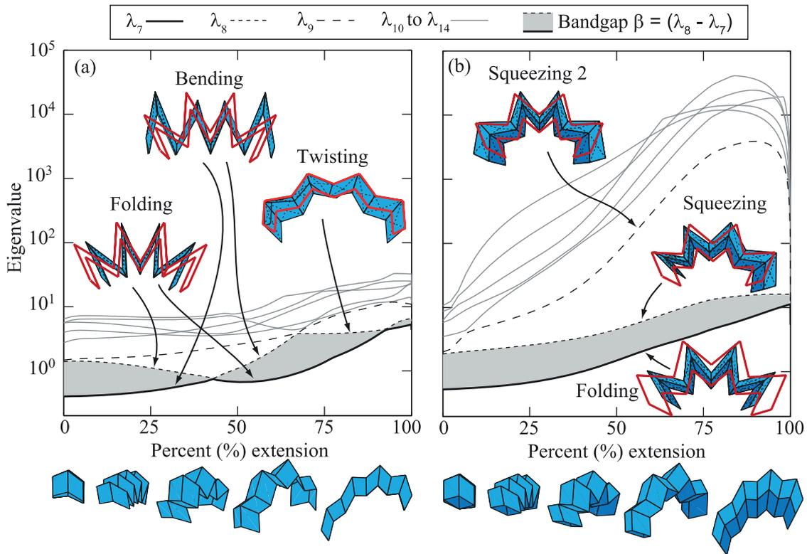
**Fig. 12.** Eigenvalues vs. configuration (% extension) of (a) a curved eggbox form and (b) a tube with the top section identical to (a). The deformation modes of the eggbox are more flexible than the tube and switch at different configurations. The tube has a continuous bandgap for different configurations indicating that it requires less energy to deploy the structure than to deform it in other ways (e.g. twisting).
