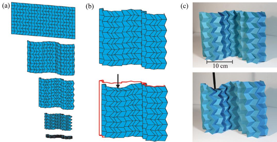
**Fig. 1.** A Miura-ori pattern with a modified curved geometry (Gattas et al., 2013). (a) Folding kinematics of the origami. (b) and (c) Initial (top) and deformed (bottom) shapes of the origami from a point load applied at the top, while the bottom of the structure is restrained vertically. (b) structural simulation with the bar and hinge model and (c) physical model of the origami.
