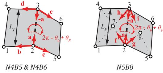
**Fig. 8.** Placement of rotational hinges to capture the fold line stiffness. The rotational constraints for the N5B8 model includes only the central nodes of the panel and thus removes the ambiguity between fold and panel bending for large displacement analyses.
