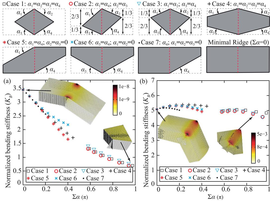
**Fig. A.17.** Influence of panel skew on bending stiffness. The panels with different skewed configurations are quantified by  $\Sigma\alpha = \alpha_1 + \alpha_2 + \alpha_3 + \alpha_4$ . Normalized bending stiffness vs. panel corner geometry ( $\Sigma\alpha$ ), for (a) small displacement bending ( $\theta_b = 1^\circ$ ) and (b) large displacement bending ( $\theta_b = 70^\circ$ ). Skew has an influence on the bending stiffness for small displacements, but not for large displacements.
