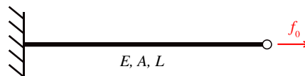
FIGURE F1 The one-bar truss example [Colour figure can be viewed at wileyonlinelibrary.com ]
