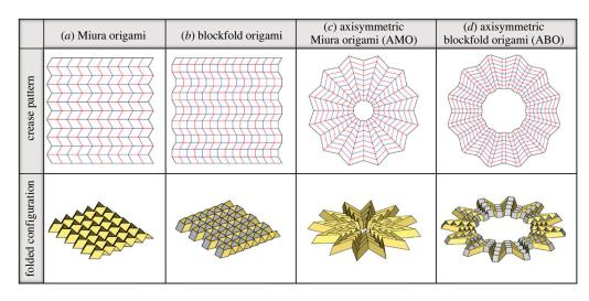
**Figure 1.** The crease patterns and folded configurations of (*a*) Miura origami, (*b*) blockfold origami, (*c*) axisymmetric Miura origami and (*d*) axisymmetric blockfold origami. The mountain and valley creases are coloured in red and blue, respectively.
